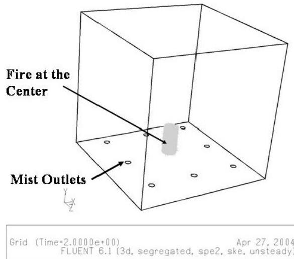
**Figure 2: Configuration of NanoMist discharge outlets on the floor of test compartment**
