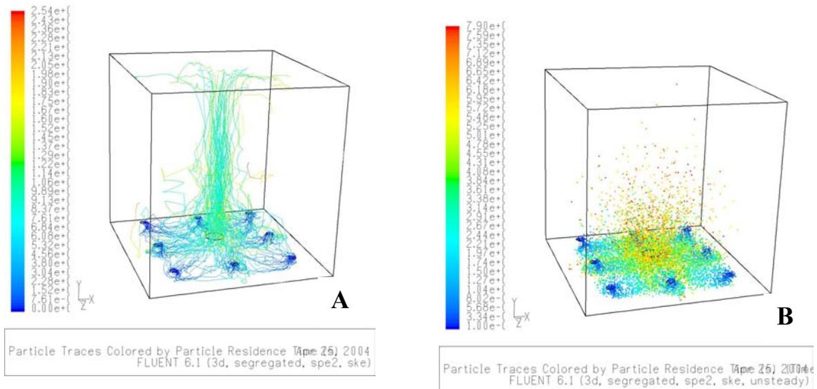
**Figure 5: A) Stochastic droplet trajectories of inert droplets, and B) droplet trajectories with vaporization.**
