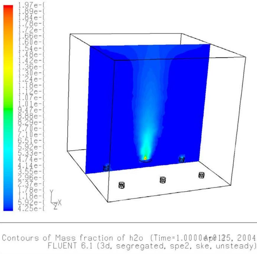
**Figure 7: Water vapor mass fraction at t=10 s. The peak value of mass fraction is 0.19**
