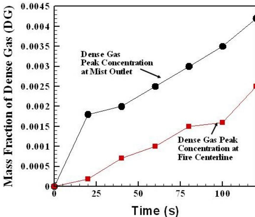
**Figure 9: Comparison of Dense Gas (DG) concentration at the mist discharge location and at the fire centerline. The concentration of dense gas is about 50% at 2 minutes.**
