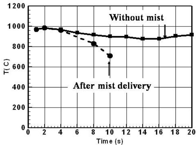
**Figure 8: Centerline peak temperature of reference fire and fire with NanoMist injection**
