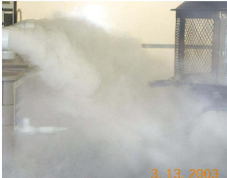
**Figure 1: A dense gas-like NanoMist water mist dispersion inside a room**
