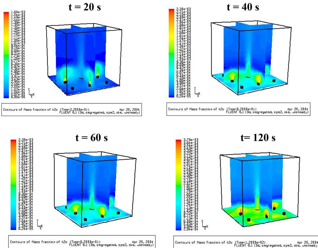
**Figure 10: Mass fraction contours of dense gas (DG) at various time intervals.**
