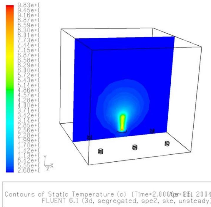
**Figure 3: Temperature ( $^{\circ}\text{C}$ ) contours of fire at  $t=2$  s. The peak temperature is  $984^{\circ}\text{C}$**
