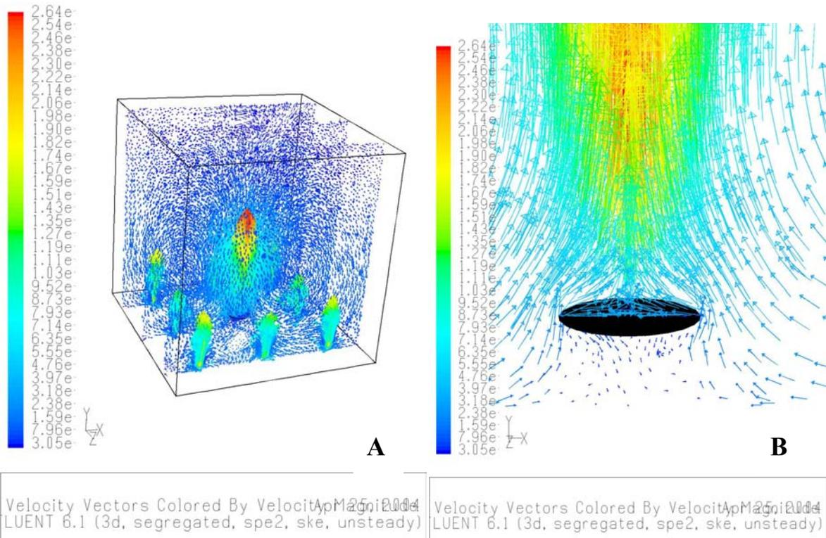
**Figure 4: A) Velocity vectors (m/s) inside the compartment and B) velocity vectors (m/s) near the firebase, a close-up view**
