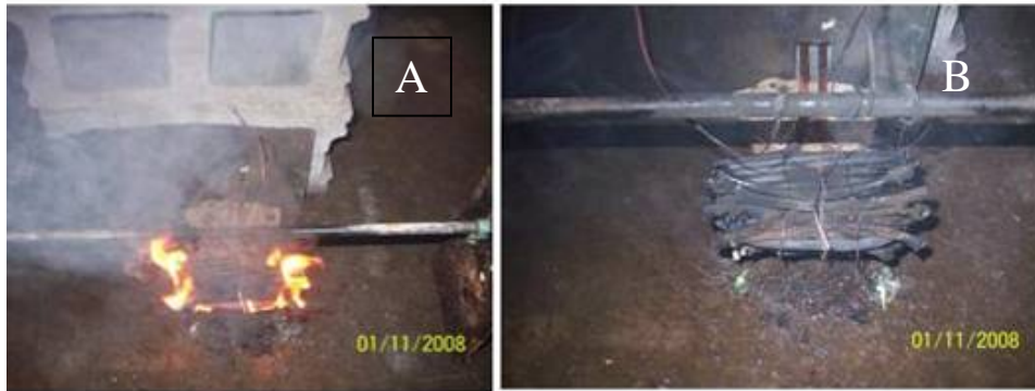
Figure 5: A. Cable bundle on the energized heater and thermocouples above it: B. Cable bundle after extinguishment of fire
