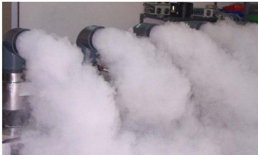
Figure 4B: NanoMist® ultra fine water mist generators
